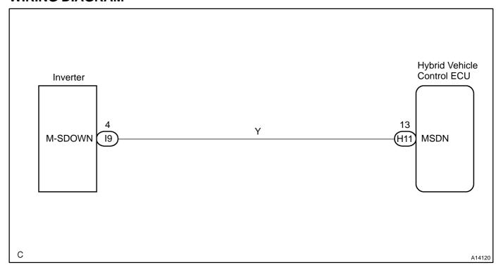
1 Check for open, short and +B short in wire harness between HV ECU MSDN terminal and converter & inverter assembly M-SDOWN terminals (See page IN-41).
