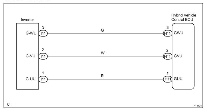
1 Check for open and short in wire harness between HV ECU terminals (GUU, GVU, GWU) and inverter terminals.
