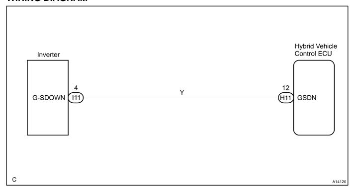
1 Check for open, short and +B short in wire harness between HV ECU GSDN terminal and converter & inverter assembly G-SDOWN terminals (See page IN-41).
