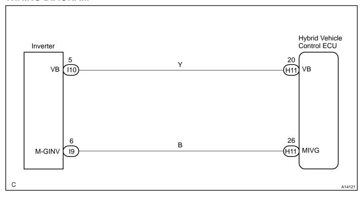
1 Check for open, short and +B short in wire harness between HV ECU VB and MIVG terminals and converter & inverter assembly VB and M-GINV terminal (See page IN-41).
