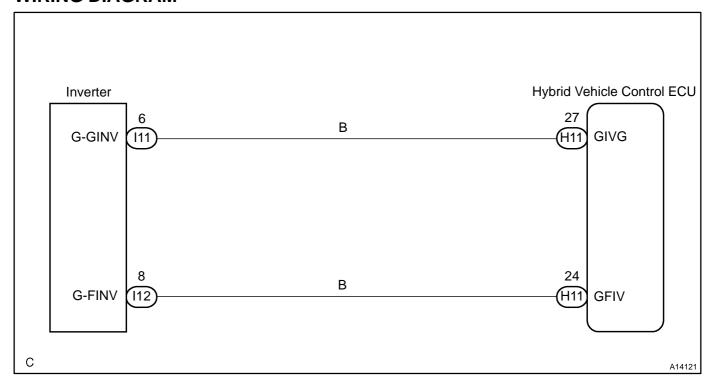
1 Check for open, short and +B short in wire harness between HV ECU GFIV and GIVG terminals and converter & inverter assembly G-FINV and G-GINV terminals (See page IN-41).
