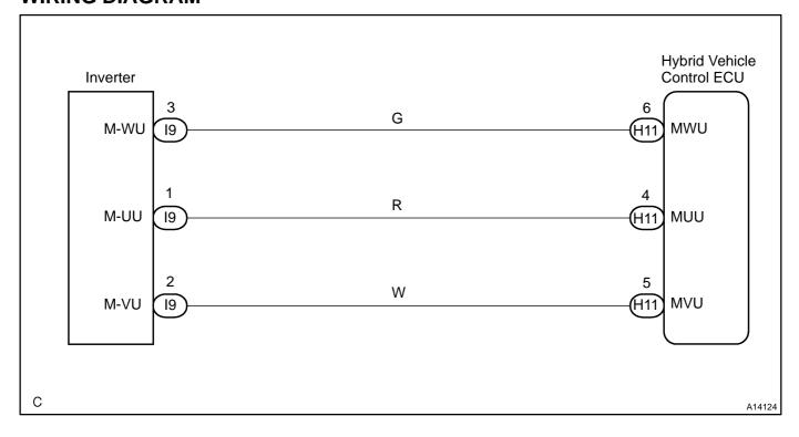
1 Check open and short in wire harness between HV ECU terminals (MUU, MVU, MWU) and inverter terminals.
