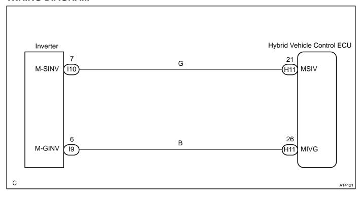
1 Check for open, short and +B short in wire harness between HV ECU MIT and MIVG terminals and converter & inverter M-INVT, M-GINV terminals (See page IN-41).
