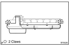
(b) Disengage the 2 claws and then remove the combination meter cover No.2.
