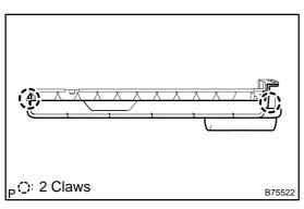
(b) Disengage the 2 claws and then remove the combination meter cover No.1.
