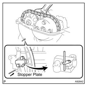
(f) Insert a 3.0 mm (0.118 in.) diameter bar into the hole of the stopper plate with the stopper plate of the chain tensioner lifted down and locked.
