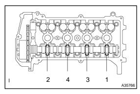
(I) Remove the camshaft bearing caps No. 2 in the sequence shown in the illustration.
