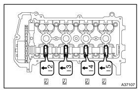
(u) Check the front marks and numbers on the bearing cap No. 2, then tighten the bolts uniformly in several steps in the sequence shown in the illustration.
