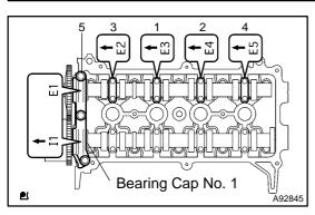
(y) Check the front marks and numbers on the bearing caps No. 1 and No. 2, then tighten the bolts uniformly in several steps in the sequence shown in the illustration.
