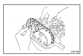
(x) Temporarily tighten the camshaft timing chain with the bolt.
