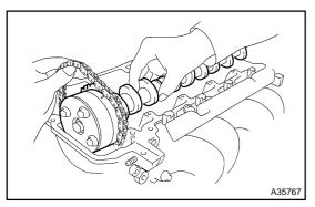
(m) Hold the timing chain by hand, then remove the camshaft.
