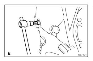
(b) Using 8 mm socket hexagon wrench, remove the service hole screw plug.
