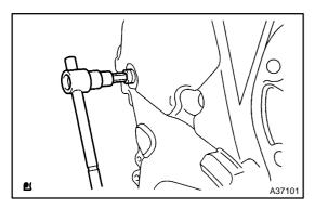
(ae) Apply adhesive to the 2 or 3 threads of the service hole screw plug bolt end.
