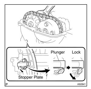
(e) Keeping the adjustable wrench installed, remove the screwdriver with the plunger pushed.
