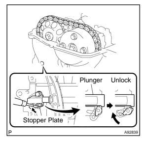
(c) Insert a screwdriver into the service hole of the chain tensioner to hold the stopper plate of the chain tensioner upward.
