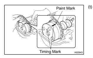
Hold the chain as illustrated, then install the camshaft and camshaft timing gear assembly so that the paint mark of the chain and the timing mark of the camshaft timing gear assembly are aligned.
