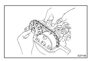
(k) Remove the bolt when the camshaft No. 2 is lifted slightly, then remove the camshaft No. 2 and camshaft timing gear.
