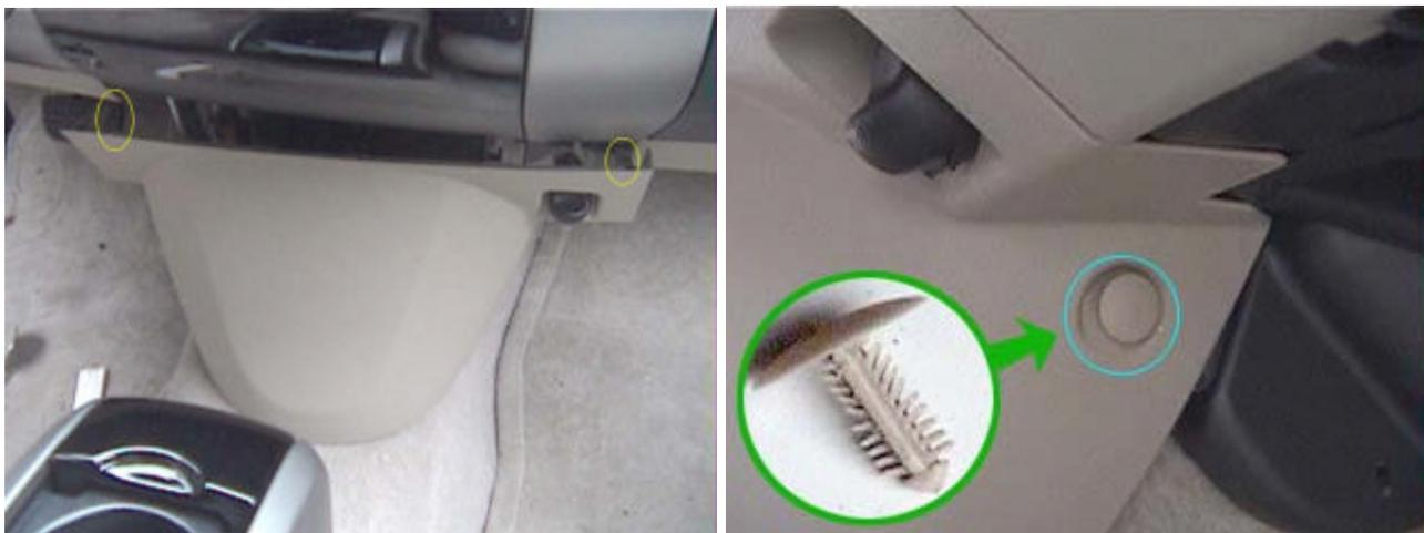
Once you get the fastener pulled out, the panel is held on by two neon-yellow snaps circled in yellow in the left picture, above. To get the snaps out, you can get one hand behind each side of the panel and just pull it firmly.
