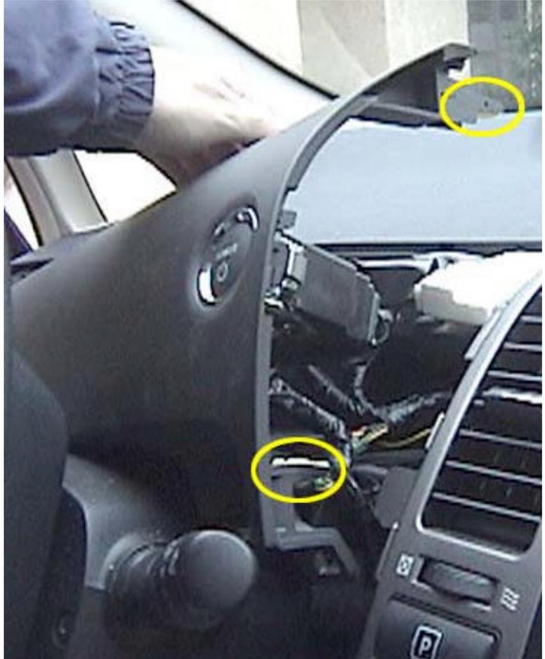
Now, you can finally remove the silver vent to the left of the stereo (outlined in blue in the upper picture to the right). It is held on by 5 snaps (circled in yellow). This panel is much easier to remove than the other vents because you can get your fingers behind it on the left. The shift knob is not attached to this panel and will slip out through a circular hole.
